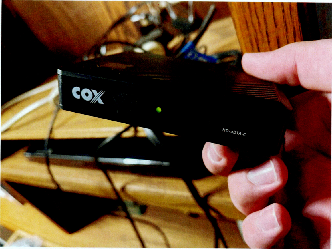
Figure 4: Cox Cable Box Displaying Green Light
